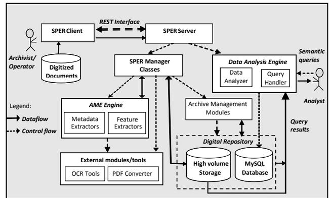
Figure 1. SPER system architecture.
